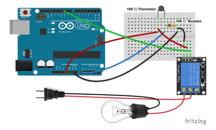
Identify the hot power wire (red wire in the diagram above) in the cord leading to the light bulb and make a cut. Connect the side leading to the light bulb to the NO terminal of the relay, and the side leading to the plug to the C terminal. This way the relay is on the hot side, and current is switched before it reaches the light bulb. It's dangerous to put the relay on the neutral wire, since if the device fails current can still fault to ground when the relay is off.
